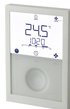
The controller connects via a cable to the controller terminal board. Dimensions: w. 125 x h. 90 x d. 32 [mm] The controller is intended for wall mounting. IP30.
